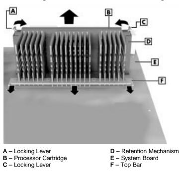
Removing the Pentium II Processor Cartridge
